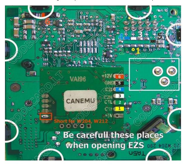
Remove from EZS board SMD part marked with red "X". With short, good isolated wire connect **CANEMU** to EZS board according picture: 1-1 (C1H), 2-2(C1L), 3-3(C2H), 4-4(C2L), 5-5(GND), and 6-6 (+5V).
