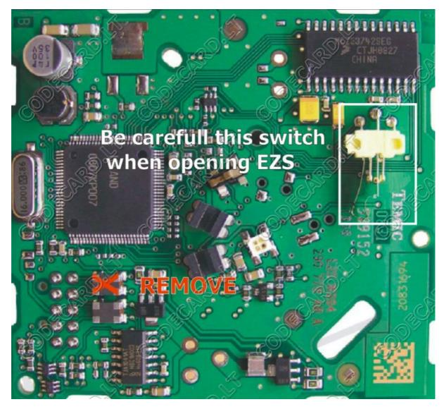
After connection insulate **CANEMU** board with heat shrink or insulation tape. Put it carefully to EZS casing.
