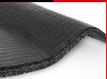
**STP VBT** – a sheet multilayer material. The material is a multilayer combination that consists of a foamed polyethylene and duplicated facial layer (it is a sheet on the base of polymer-bitumen composition covered by a transparent film). The backing of the material is a uniform foamed polyethylene with smooth or rugged surface.
